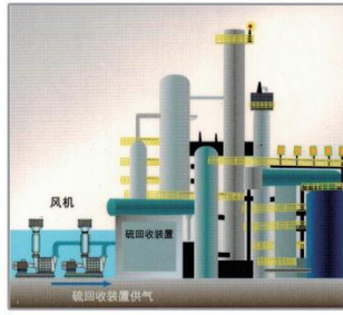
脱硫系统 Esulfurization equipment system
